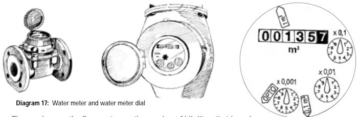
The numbers on the flow-meter are the number of kilolitres that have been pumped.
