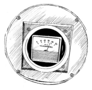
**Diagram 8:** Gauge showing that the probe is not in the water
